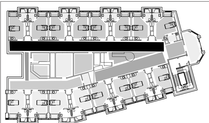
Figure 6. Integration- n analysis of the convex spaces of a hypothetical MSU. Higher integration values are indicated by darker lines.
